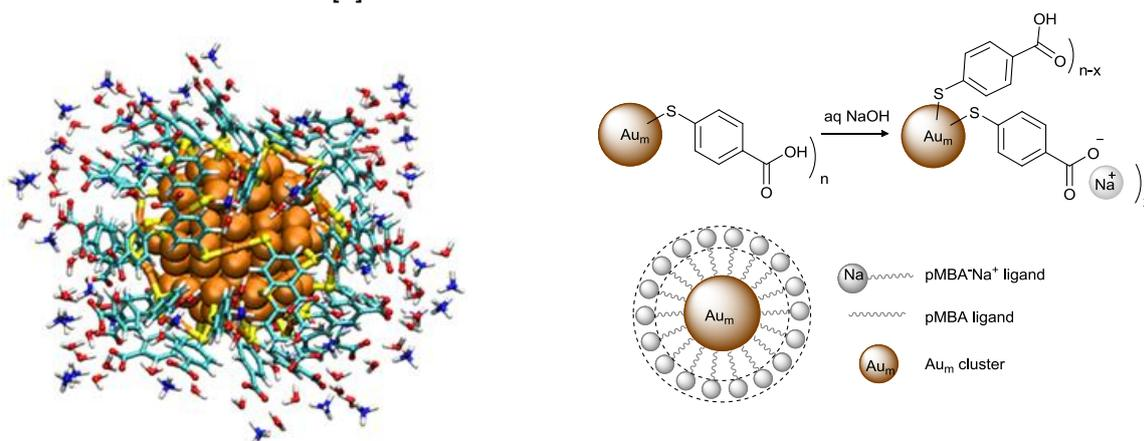
Scheme 1: Left: A model cluster of  $Au_{102}(SR)_{44}$  built using computationally relaxed  $pMBA^{-} \cdots 2H_2O \cdots NH_4^{+}$  complex as a ligand. Right: Schematic presentation of the  $Au_m(pMBA)_n$  clusters as their sodium salts in aqueous NaOH solution highlighting the effect of sodium counter cation on the hydrodynamic diameter (----) of the cluster.
