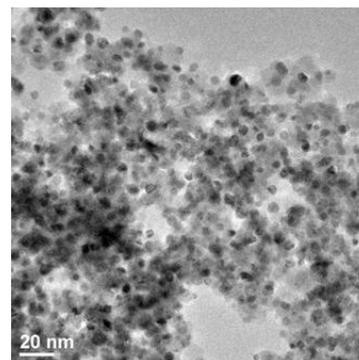
**Fig. 1.** TEM image of Ag@Pd/TiO<sub>2</sub> catalysts prepared by microwave heating.
