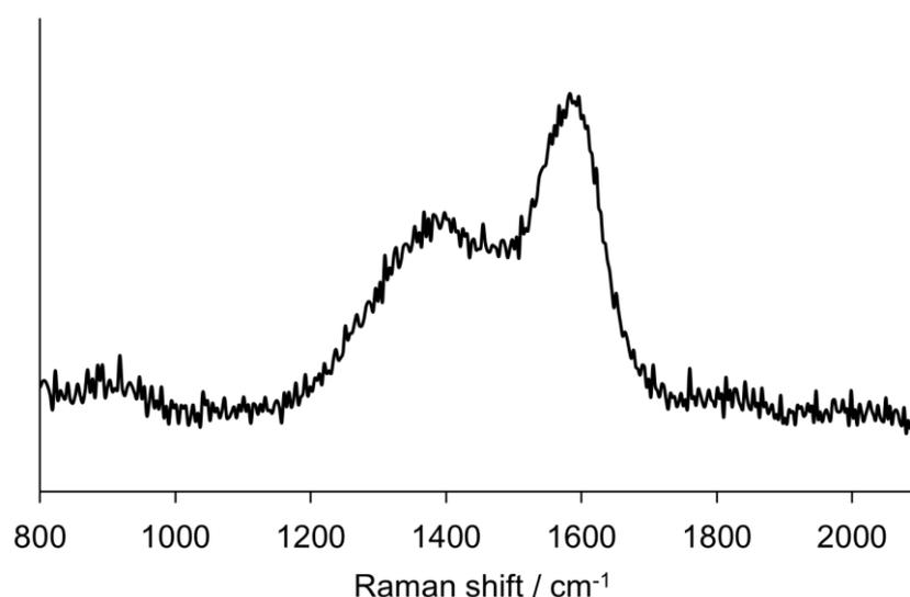
Figure: Raman spectrum of genuinely amorphous carbon. Copper acetylide nano materials could be carbonized at a temperature of 200°C.
