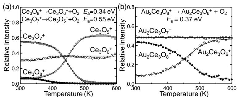
Figure 2. Relative intensities of (a)  $\text{Ce}_3\text{O}_{5-8}^+$  and (b)  $\text{Au}_2\text{Ce}_3\text{O}_{6-8}^+$  as functions of heating temperature.
