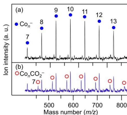
Figure 1. Mass spectra of Co<sub>*n*</sub><sup>-</sup> (a) before and (b) after the reaction with CO<sub>2</sub>.
