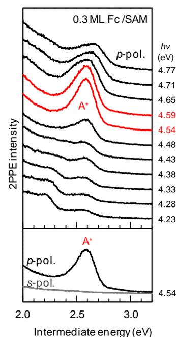
Figure 1. Photon energy ( $h\nu$ ) and polarization dependent 2PPE spectra of 0.3 ML Fc on SAM.
