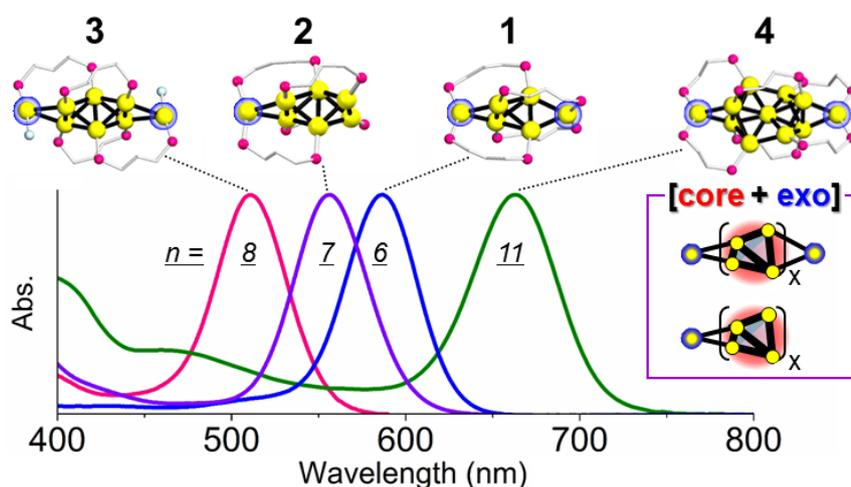
**Figure 1.** Skeletal structures and absorption spectra of  $Au_n$  clusters ( $n = 6, 7, 8, 11$ ; **1 - 4**). Inset shows [core+exo] motif, in which one or two exo Au atoms are attached to centered polyhedral Au cores.
