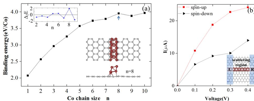
Figure. (a) Binding energy per Co atom as a function of the Co chain size (n). The insets are second difference  $\Delta_2 E(n)$  as a function of n. (b) Spin-dependent I-V curves for the hybrid system.
