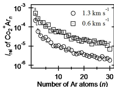
Fig. 1. Size distributions of  $\text{Co}_2^+\text{Ar}_n$ . Intensities were normalized to unreacted  $\text{Co}_2^+$ . The broken lines are fitting curves.
