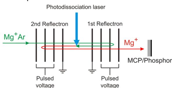
Fig. 1 Schematic diagram of the apparatus
