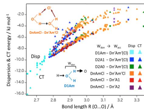
Figure 2. The correlation between the bond length  $R_{\text{O}\dots\text{O}}$  of water and water vs.  $E_{CT}$  and  $E_{Disp}$  in the  $\text{Cl}^-(\text{H}_2\text{O})_n$  ( $n=3-7$ ) cluster
