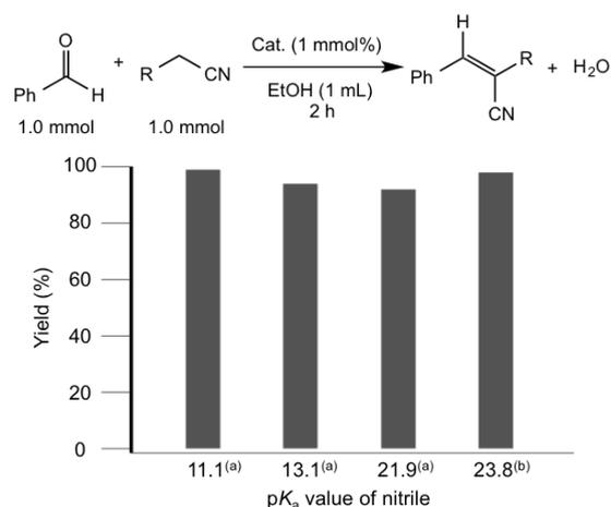
Figure 2: Knoevenagel condensation catalyzed by  $\text{TBA}_6[\text{Nb}_{10}\text{O}_{28}]$  for nitriles with various  $\text{pK}_a$  values (reaction temperature: (a)  $30^\circ\text{C}$ , (b)  $80^\circ\text{C}$ ).
