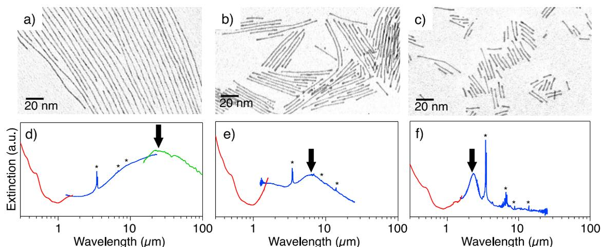
Figure 1. a)–c) Typical TEM images and d)–f) optical extinction spectra of Au UNWs and UNRs with the lengths of 370, 40, and 20 nm, respectively. The asterisks indicate vibrational peaks of OA.
