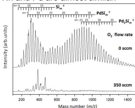
**Figure 1.** Mass spectra of Pd-Si NC cations.
