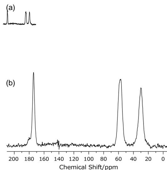
Figure 1  $^{13}\text{C}$  NMR spectra of (a) CdSe-11 and (b) CdSe-9, measured with a 1 ms contact time.
