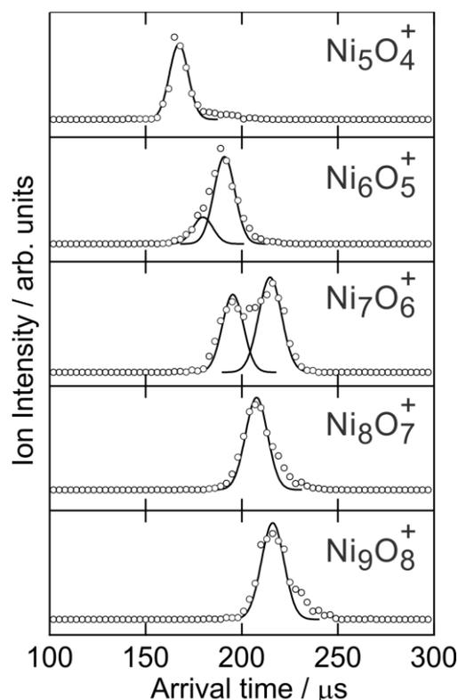
Figure 1. Arrival time distributions of  $\text{Ni}_n\text{O}_{n-1}^+$  cluster ions for  $n = 5-9$ . Open circles are the observed ion intensities, and the Gaussian curves show components of isomers.
