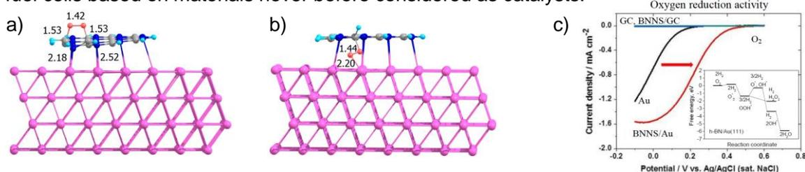
Figure 1. Optimized structures of O<sub>2</sub> adsorbed at the edge of the small h-BN island on the Au(111) surface (a) and (b). The linear sweep voltammograms of (i) bare Au, (ii) BNNS/Au, (iii) bare glassy carbon (GC), and (iv) BNNS/GC as well as free energy diagram for ORR on the h-BN/Au(111) (c).
