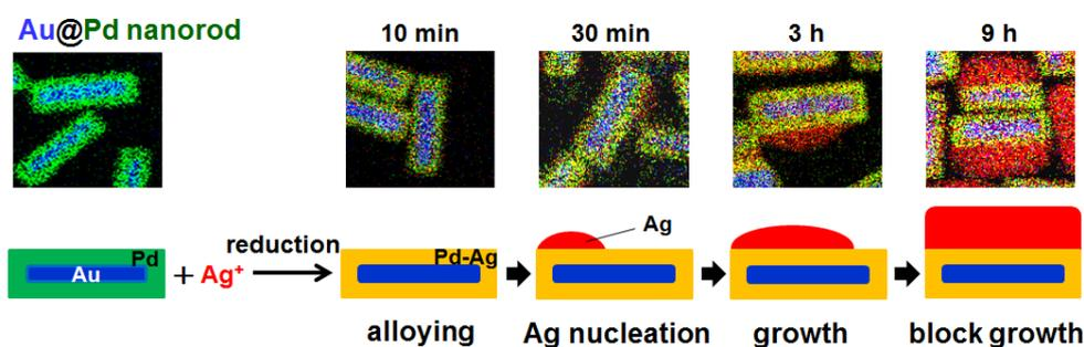
Fig. 1. TEM-EDS images and growth mechanism of rectangular Au@PdAg@Ag nanorod.
