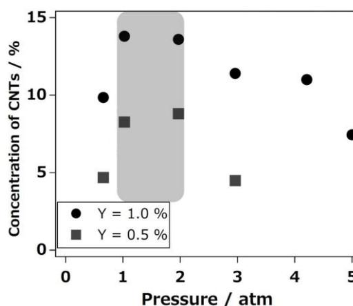
Fig. 1 Pressure Dependence of CNT concentrations obtained by TGA
