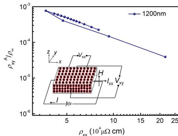
Fig. 1 The plot of  $\log(\rho_{xy}^A / \rho_{xx}) - \log \rho_{xx}$  for the film with  $t_a=1200$  nm.
