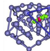
Fig. 1 The most stable H diffusion path in Pd<sub>55</sub>
