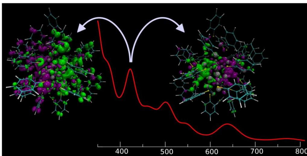
*Figure 1:* The plasmon like nature of Ag<sub>44</sub>SR<sub>30</sub><sup>4-</sup> upon excitation around 400 nm is shown. The counter interacting field of the silver-d states (right) and ligand+silver-s states (left) can be seen from the induced density as well as the contribution of the phenyl rings to the plasmonic peak.
