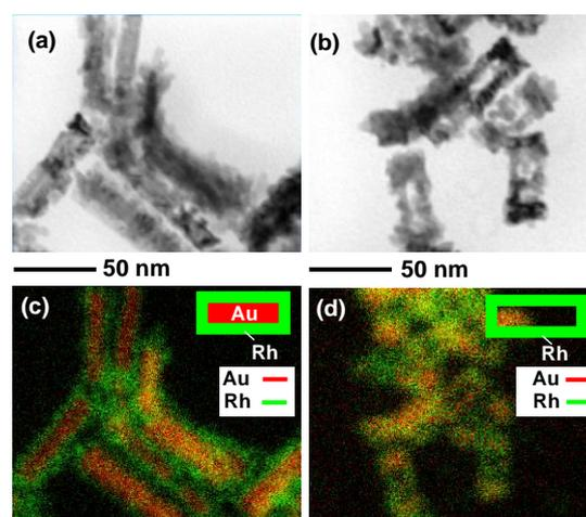
**Figure 1.** TEM images of (a) Au@Rh NRs and (b) Rh nanoframes. TEM-EDS images of (c) Au@Rh NRs and (d) Rh nanoframes.
