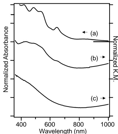
Figure.1 (a) UV-vis absorption spectrum of  $\text{Ag}_{44}(\text{MBA})_{30}$ , and diffuse reflectance spectra of  $\text{Ag}_{44}(\text{MBA})_{30}/\text{Al}_2\text{O}_3$  (b) before and (c) after calcination.
