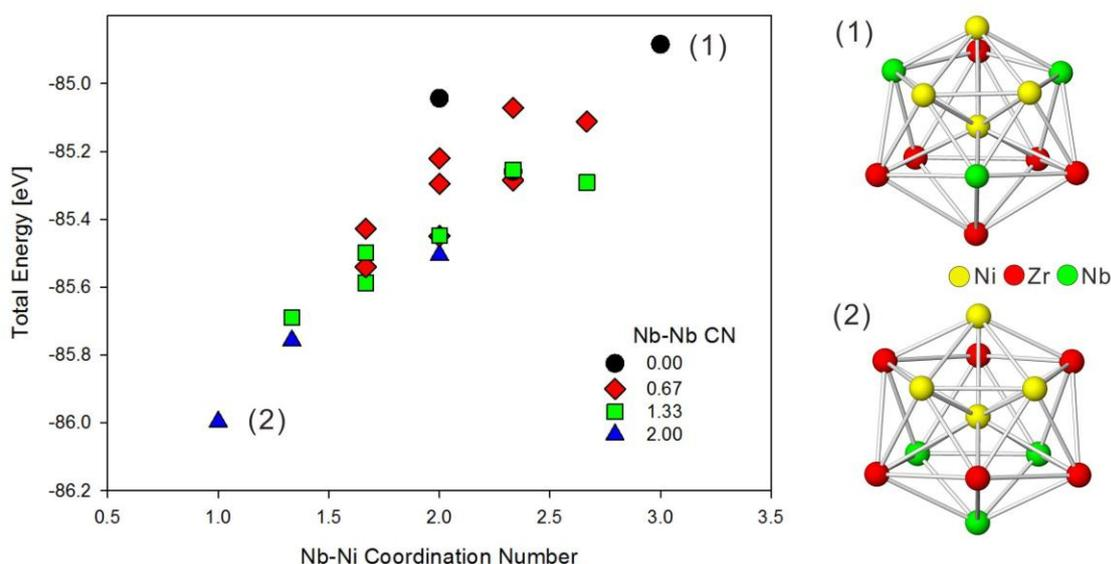
Fig.1 Nb-Ni coordination number dependence in total energy of  $\text{Ni}_4\text{Zr}_6\text{Nb}_3$  icosahedral clusters and optimized structures of two clusters (1) and (2).
