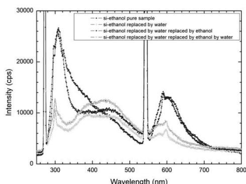
Figure 1. Fluorescence spectra of silicon nano clusters in ethanol and water. The solid symbols show fluorescence spectra for silicon clusters in ethanol, with the peak position at 320 nm. As the sample dried and dissolved into the water, the peak position shifted to 440 nm as is seen in the empty symbols.
