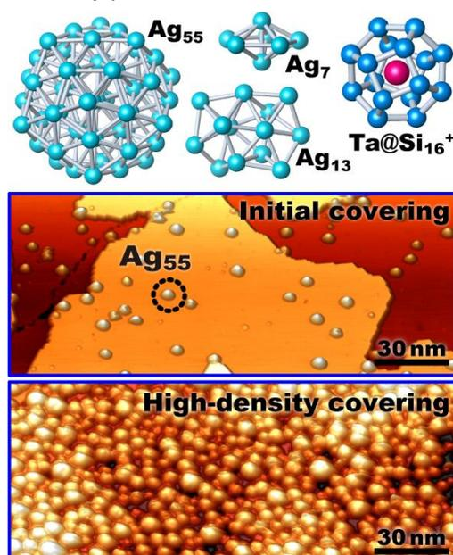
**Figure 1.**  $\text{C}_{60}$  thin films (upper) sparsely and (lower) densely covered with  $\text{Ag}_{55}$
