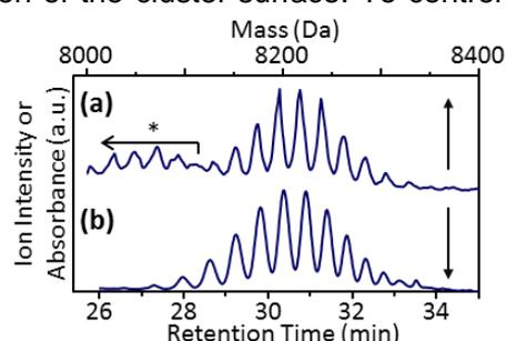
Figure 1. Comparison of (a) MALDI-MS and (b) linear-gradient chromatogram of as-prepared cluster..
