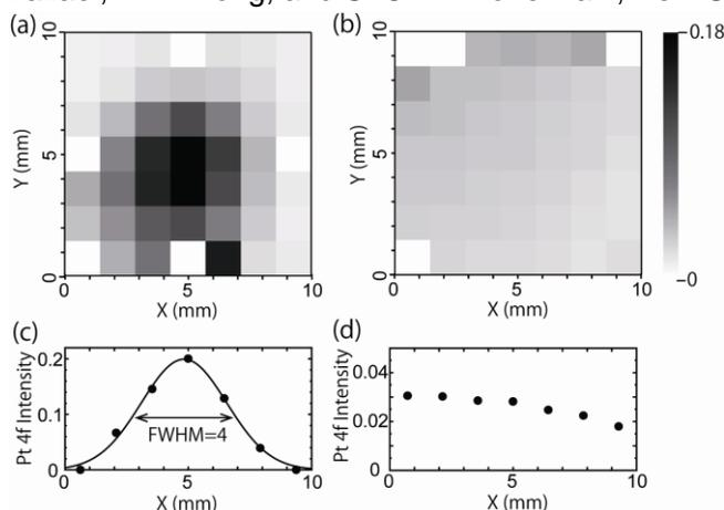
Fig. 2. Pt 4f intensity of (a) Pt<sub>4</sub>/TiO<sub>2</sub>(110) prepared without deflector, and (b) Pt<sub>15</sub>/TiO<sub>2</sub>(110) prepared with deflector. (c) Line profile at Y=5 mm of fig. 2(a), and (d) that of fig. 2(b).
