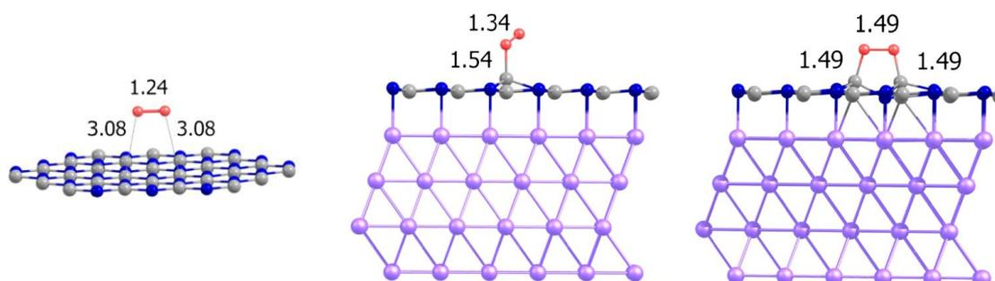
Figure 1. Optimized structure of the molecular oxygen physisorbed on a free h-BN monolayer (left) and chemisorbed on the h-BN/Ni(111) surface in on top (middle) and bridge (right) configurations.
