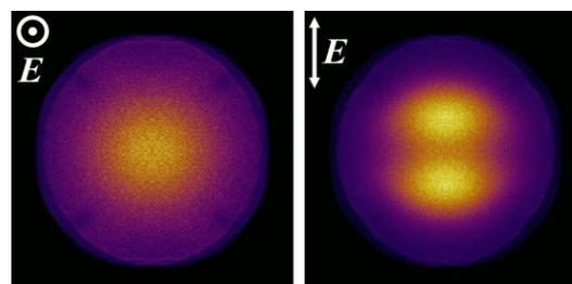
Fig. 2 Observed images of fragment ion  $\text{Mg}^+$  for  $\mathbf{E} \parallel \mathbf{Z}$  (left),  $\mathbf{E} \perp \mathbf{Z}$  (right)
