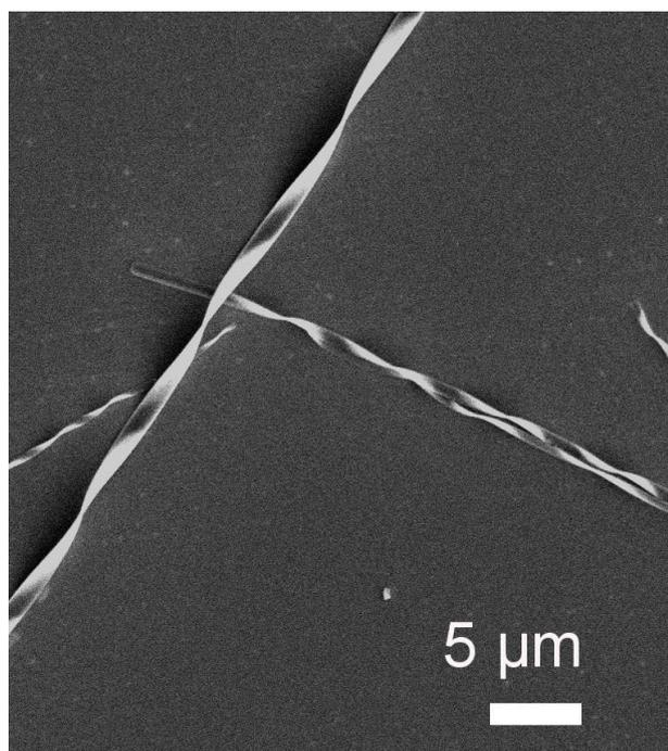
Figure: Scanning Electron Microscopy (SEM) image of twisted silver tolylacetylide.
