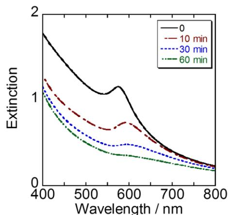
Figure 1. Extinction spectra of copper nanoparticles for air-exposure time.
