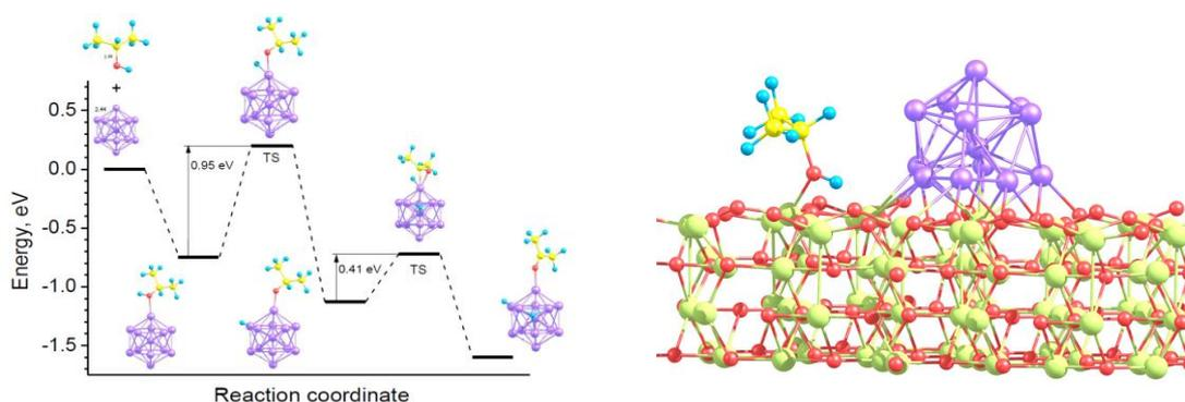
Figure 1. Energy diagram for dehydrogenation of C<sub>3</sub>H<sub>8</sub>O on the free Ni<sub>13</sub> (left) and adsorption of isopropanol in the vicinity of Ni<sub>13</sub> cluster supported on  $\Theta$ -Al<sub>2</sub>O<sub>3</sub>(010) surface (right).
