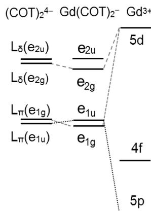
Fig. 1: Qualitative orbital interaction scheme of  $\text{Gd}(\text{COT})_2^-$
