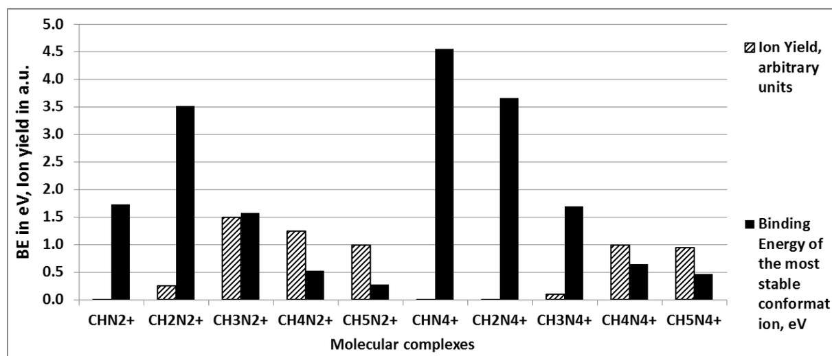
Fig. 1 Ion yield and binding energy values of monocarbon molecular complexes
