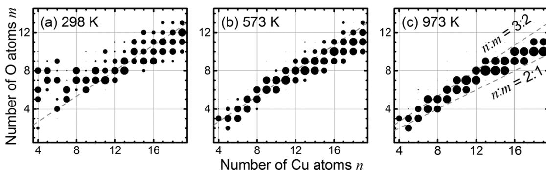
Figure 1 Mass abundance of  $\text{Cu}_n\text{O}_m^+$  clusters: (a) without heating treatment, (b and c) after heating treatment. Area of each bubble is proportional to the normalized intensity ( $\text{Cu}_n\text{O}_m^+ / \sum_m \text{Cu}_n\text{O}_m^+$ ).
