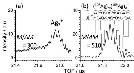
Fig. 2. TOF mass spectra of  $\text{Ag}_7^+$  measured with meshes on all the electrodes (a), and on EL1 only (b). The peaks marked with asterisks are ringing noise.
