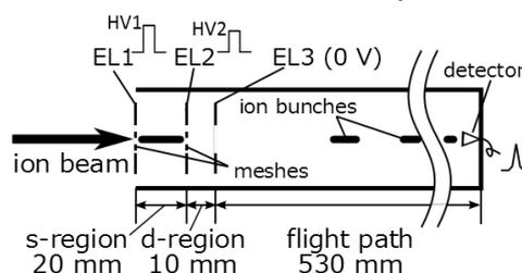
Fig. 1. A schematic view of the present time-of-flight mass spectrometer.
