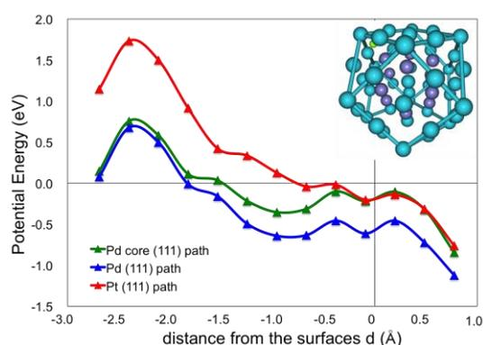
Fig. 1 H-absorption potential energy curves for  $\text{Pd}_{55}$ ,  $\text{Pt}_{55}$ , and core-shell type  $\text{Pd}_{13}\text{Pt}_{42}$  shown in r.h.s.
