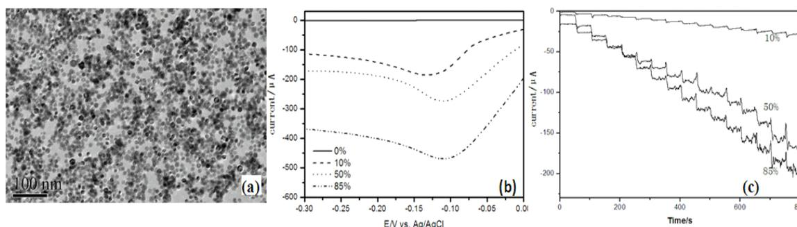
Fig.1. (a) TEM image of the Pd clusters deposited on amorphous carbon film surface. (b) The linear sweep stripping voltammetry (LSSV) measurements of the Pd NPs/GCE with different nanoparticle coverage in 0.01M H<sub>2</sub>O<sub>2</sub> (0.05M PBS, pH=7.4) at the scan rates of 0.05V/s. (c) The amperometric responses of the Pd NPs/GCE with different nanoparticle coverage deposition times upon successive addition of H<sub>2</sub>O<sub>2</sub> into gently stirred 0.05 M PBS (pH 7.4) at  $-0.11$ V.
