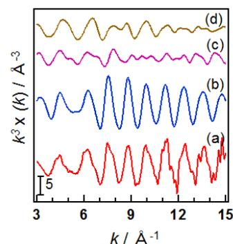
Fig. 2 Pd-K edge EXAFS spectra of  $\text{Au}_{24}\text{Pd}_1(\text{SC}_{12}\text{H}_{25})_{18}$  obtained by (a) experiment, (b)  $\text{Pd}_C$ , (c)  $\text{Pd}_S$ , and (d)  $\text{Pd}_O$  models.
