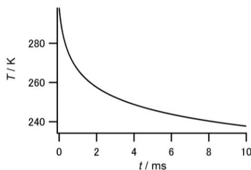
**Figure 2.** A cooling rate calculated for a water droplet with 74- $\mu\text{m}$  in diameter at 0 Pa
