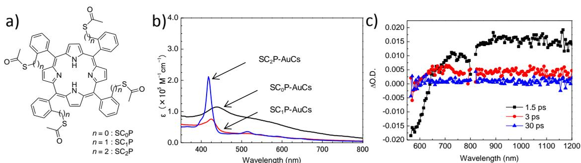
Fig.1 a) structure of porphyrin derivatives ( $SC_nP$ ,  $n = 0 \sim 2$ ), b) UV-vis-NIR absorption spectra of  $SC_nP$ -coordinated AuC, c) TA spectra of  $SC_0P$ -coordinated AuC.
