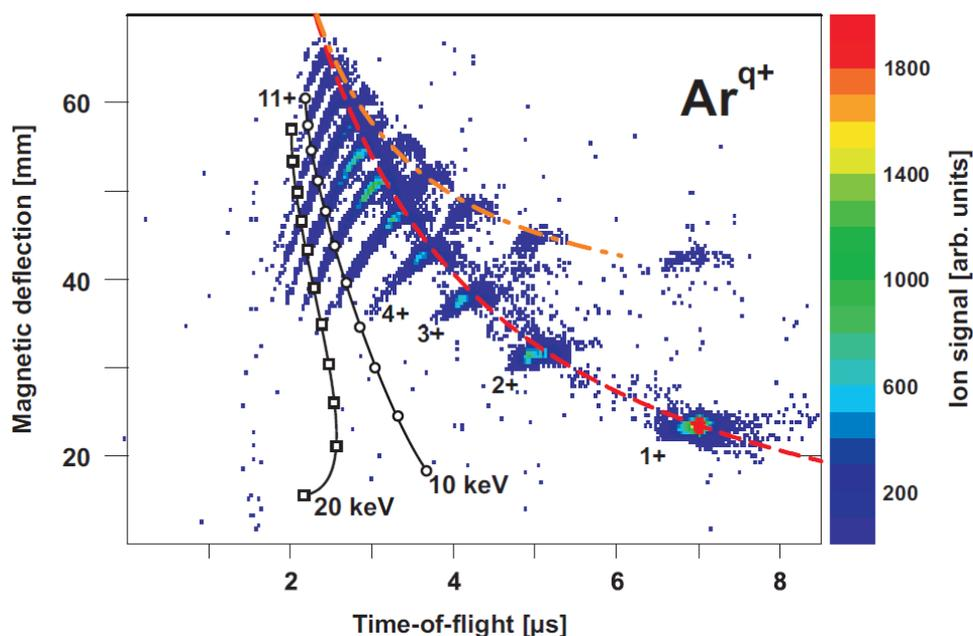
Figure 1: Magnetic deflection time-of-flight imaging spectrum of the Coulomb explosion of argon clusters ( $N=1000$ ) exposed to intense femtosecond laser pulses ( $\tau_L = 110$  fs,  $I_L = 2.3 \times 10^{15}$  W/cm<sup>-2</sup>, double pulse delay  $\Delta t = 500$  fs).
