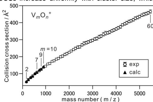
Fig.1 Experimental ( $m = 2-60$ ) and theoretical ( $m = 2-10$ ) CCSs of  $V_mO_n^+$ .
