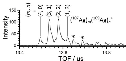
Fig. 3. A TOF mass spectrum of  $\text{Ag}_3^+$  extracted from a linear ion trap.
