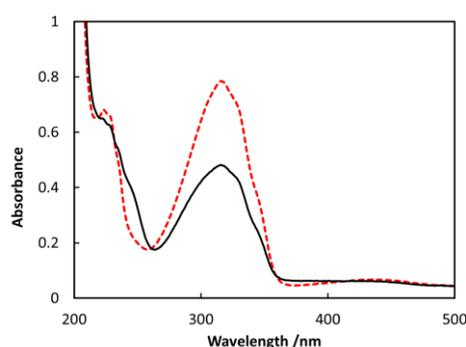
Figure 1. The absorption spectrum for the sample before (red dashed line) and after (black solid line) visible light irradiation for 4 hours.
