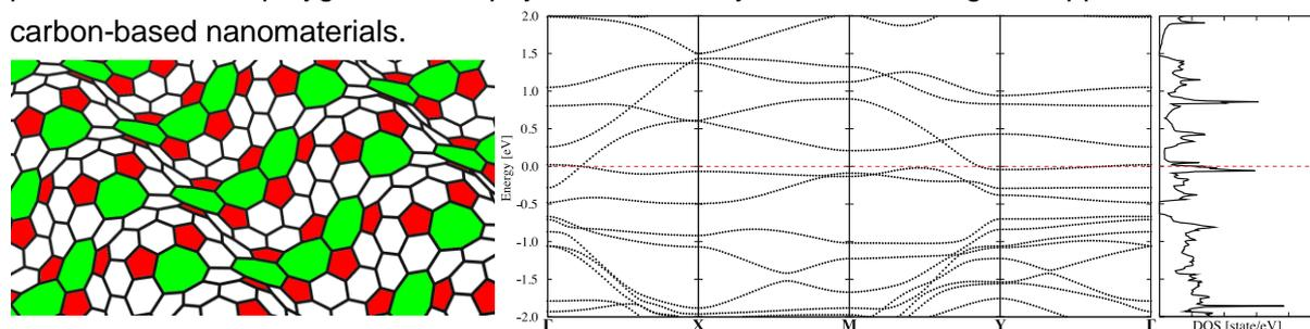
Fig.1 Geometrical structure, band structure, and DOS of corrugated graphene (Fermi energy is set at 0.0 eV)
