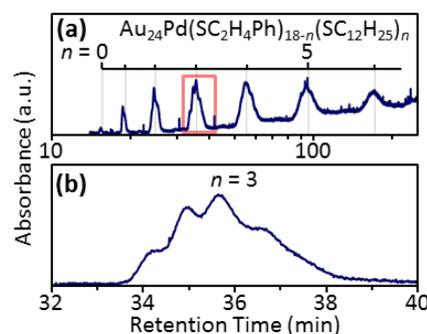
Figure 3. (a) Linear-gradient Chromatogram and (b) expanded chromatogram of squared area in (a).
