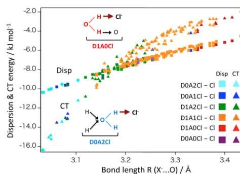
Figure 1. The correlation between the bond length  $R_{\text{X}\dots\text{O}}$  of halogen and water vs.  $E_{CT}$  and  $E_{Disp}$  in the  $\text{Cl}^-(\text{H}_2\text{O})_n$  ( $n=3-7$ ) cluster
