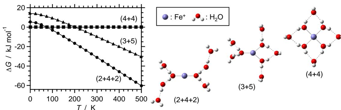
Fig. Optimized geometries for three isomers of  $\text{Fe}^+(\text{H}_2\text{O})_8$  and free energy of (2+4+2) and (3+5) relative to (4+4) as a function of temperature in the 0–500 K range.
