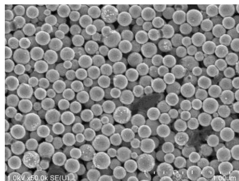
Fig. 1 Au SSMPs produced by the laser-induced melting of the source Au NPs stabilized by 0.05 mM NaCl.
