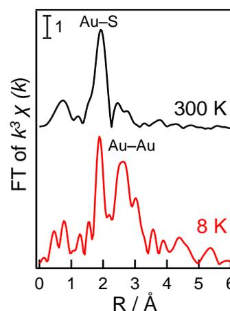
Fig. 1 Au  $L_3$ -edge FT-EXAFS spectra of  $\text{Au}_{25}(\text{SC}_2\text{H}_5\text{Ph})_{18}$  at 300 K and 8 K
