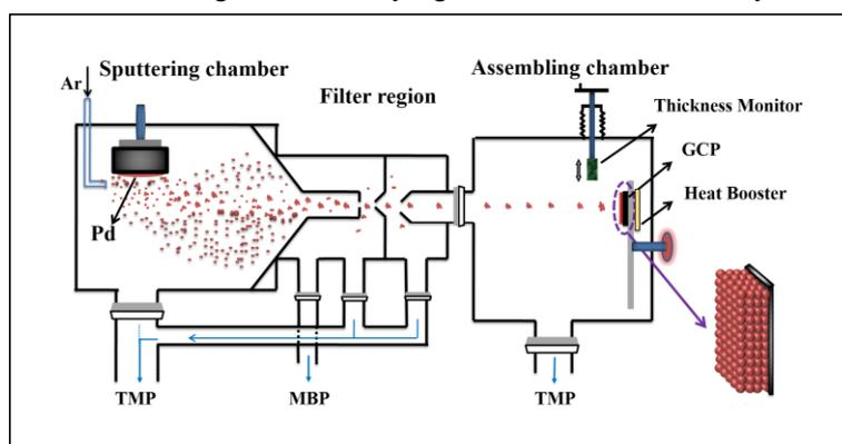
Fig. 1. Schematic diagram of Pd NC deposition process in the nanoparticle composite deposition system.
