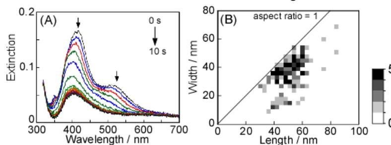
Fig. 1 Fig. 1. (A) Extinction spectral changes observed in the deposited core-shell nanorods under an applied constant potential (0.15 V vs. SCE) in the KCl solution (0.1 M). (B) size distribution of the deposited core-shell nanorods after a 10 s electrolysis. The scale bar indicates the frequencies of nanoparticles
