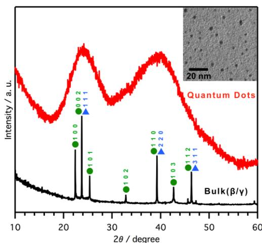
Figure. PXRD patterns of bulk silver iodide and quantum dots (inset: TEM image of silver iodide quantum dots)<sup>[2]</sup>
