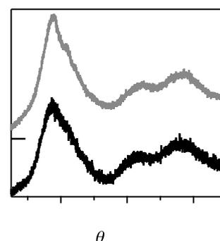
**Figure 1.** Powder XRD patterns of **1** (black) and **2** (gray). (Cu K $\alpha$ )
