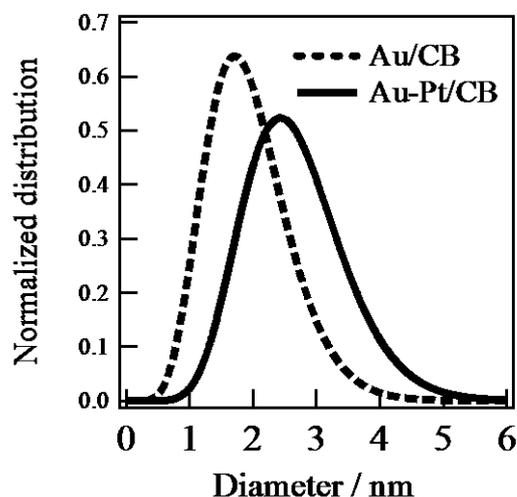
Fig. 2 The size distribution of the formed nanoparticles.
