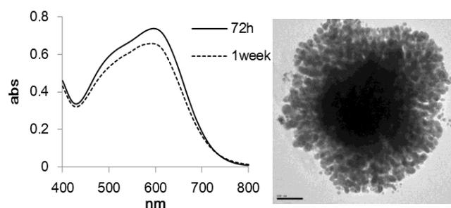
Fig. 1 Absorption of spectra (left) and TEM image (right, scale bar 100 nm) of **2a-AuNp**
