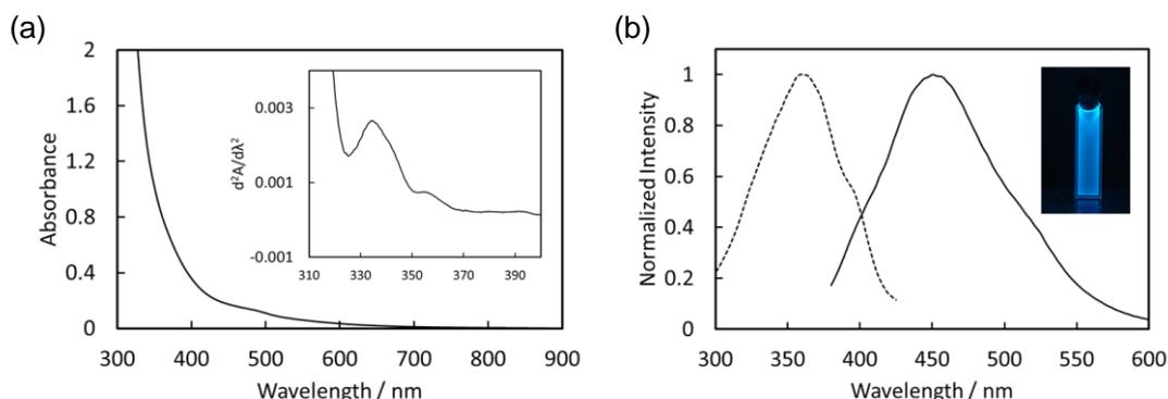
Figure 2. (a) The UV-vis and the secondary differentiation (inset) spectra of BD1-protected AuCs. (b) Excitation (dashed) and emission (solid) spectra of the AuCs. Inset shows emission under UV irradiation (365 nm).
