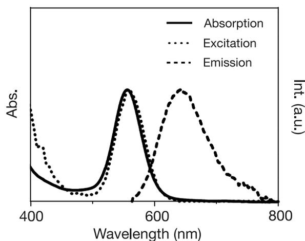
Fig.2 Absorption, emission ( $\lambda_{\text{ex}} = 555$  nm) and excitation ( $\lambda_{\text{em}} = 642$  nm) spectra of **2**.
