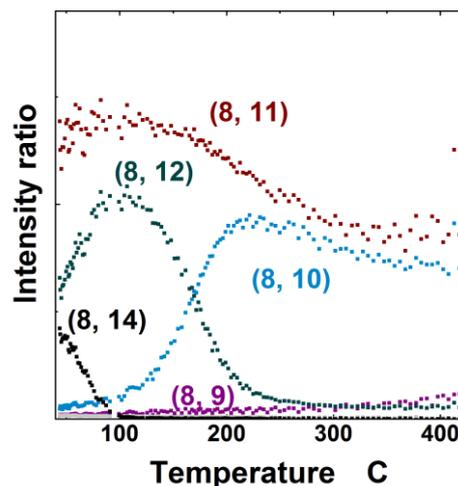
Fig. 2 Abundance ratio of  $\text{Mn}_n\text{O}_m^+$  clusters ( $n = 8$ ) increasing temperature .
