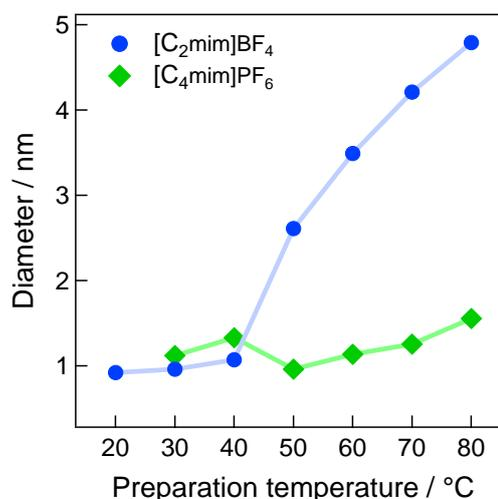
Figure 1. The size of maximum abundance in AuNPs in two ionic liquids.
