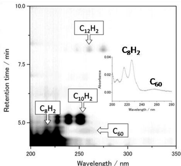
Figure 1 Two dimensional spectrum of decalin solution prepared by laser ablation in 1% propane. The inset is UV absorption spectra at retention time 4.6 min.
