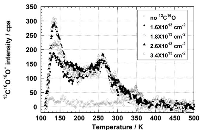
**Figure 1.** TPD spectra of  $^{13}\text{C}^{16}\text{O}^{18}\text{O}$  produced in thermal oxidation of  $^{13}\text{C}^{16}\text{O}$  by  $^{18}\text{O}_2$  catalyzed on Pt<sub>30</sub> disks bonded to a Si substrate at the various adsorption amounts of  $^{13}\text{C}^{16}\text{O}$  at the constant  $^{18}\text{O}_2$  one of  $8.5 \times 10^{-11} \text{ cm}^{-2}$ .
