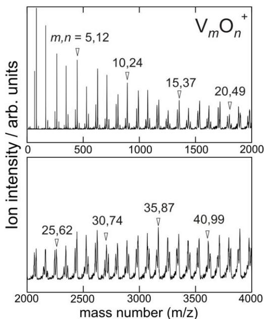
Figure 1. Cationic vanadium oxide clusters with even and odd numbered stoichiometry.
