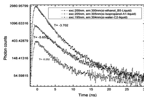
Figure 2. Lifetime of silicon nanoparticles in water (top), ethanol (middle), and isopropanol (bottom).
