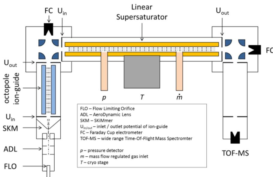
**Fig.1** Scheme of the experimental setup for heterogeneous chemistry on atmospheric nanoparticles. "TRAPS": Trapped Reactive Atmospheric Particles Spectrometer
