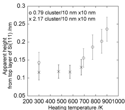
Figure 1: Temperature dependence of Apparent height of Pt<sub>30</sub> disk at two cluster density
