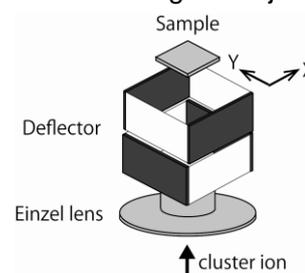
Fig. 1. Experimental set up of ion optics with deflector.
