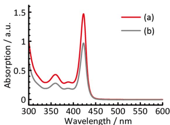
Figure 1 Absorption spectra of CdSe NPs aq. (a) just after preparation and (b) redispersed after solidification.
