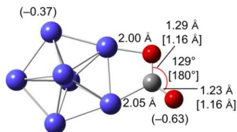
Figure 2. Optimized structure of Co<sub>7</sub>CO<sub>2</sub><sup>-</sup>. The numbers in parenthesis indicate Mulliken charge. Structure parameters of free CO<sub>2</sub> are also shown in brackets.
